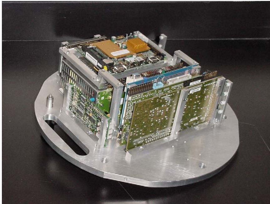
Figure 3: Fabrication of electronics compartment with electronics baseplate, electronic mounting pieces, and electronic components.
