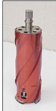
Figure 4. Modification to hydrate drill to accommodate large bore hydrate core.
