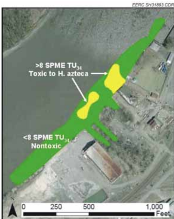
Figure 4 – Using sediment pore water PAH concentrations to delineate impacts focuses remedial design on areas of toxicity.
