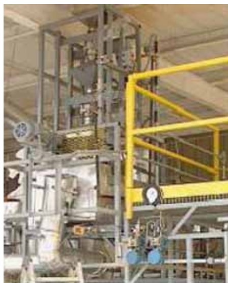
Figure 1. Pilot plant pyrolysis unit with biomass feedstack system
