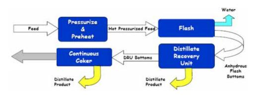
The WRITE process enables distillation of pipeline-ready heavy oil in the field rather than requiring transport to a central location as bitumen supplemented with diluents.
