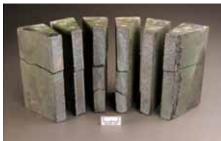
Refractory brick following exposure in the rotary kiln test: To the left are commercially produced high-chromium oxide refractories; to the right are the improved refractories
