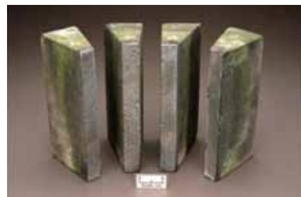
Refractory brick following exposure in the rotary kiln test: To the left are commercially produced high-chromium oxide refractories; to the right are the improved refractories
