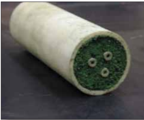
NETL-engineered thermocouple protection system for gasifier systems
