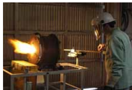
Laboratory test of refractory performance under extreme operating conditions
