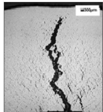
Creep failure of a tube bend as a result of cold work (strain hardening)
