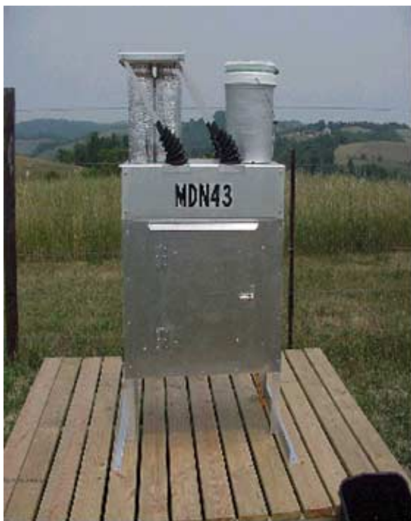
Mercury Wet Deposition Monitor near Holbrook, Greene County, PA
