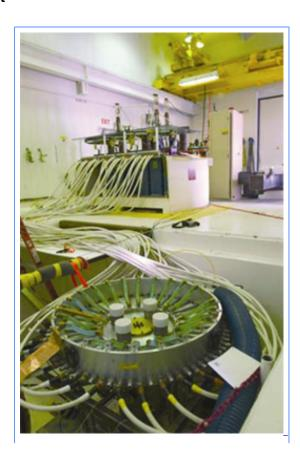
One of NSTec's Dense Plasma Focus (DPF) sources was recently relocated to Area 11 on the NTS to conduct research and development activities to enhance the country's nuclear detection capabilities. Previously, DPF used only deuterium fusion. Now it uses a deuterium-tritium gas load. Deuterium-tritium fusion creates controlled, higher-powered reactions that can be used to calibrate neutron yield detectors.
