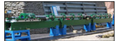
Once fully assembled, the NTS Powder Gun will be approximately 20 meters (65 feet) in length.
