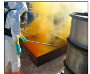
The reaction with the neutralizing agent prepares the nitric acid for disposal.
