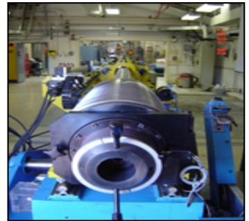
This perspective shows the breech end of the gas gun, down the barrel, to the secondary containment chamber. JASPER provides a way to generate and then measure data that is crucial to certify the safety of the stockpile. JASPER supports a key NSTec vision -- to transform the Nevada Test Site into the preferred place to conduct high-hazard experiments to support America's security.
