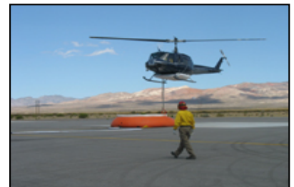
A helicopter, guided in by the NTS Fire & Rescue Water Supply Officer, prepares to refill its 350-gallon belly tank. The snorkel pump hangs below a 5,000-gallon water vessel or "pumpkin." Upon filling the tank, the helicopter continues to attack fire hot-spots during the Calico Hills Fire in 2006.
