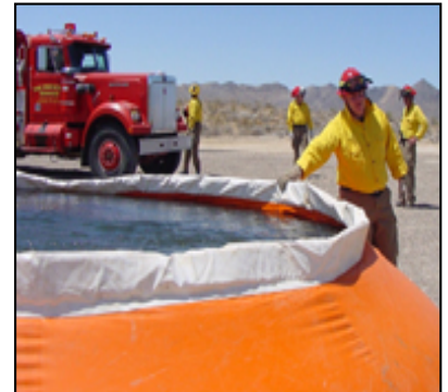
NTS Fire and Rescue firefighters fill a pumpkin-like, 5,000-gallon water dip tank with life saving water from the fire truck.
