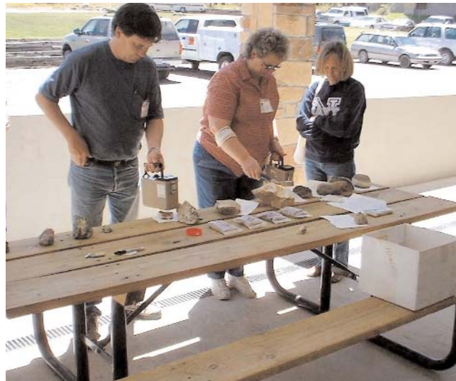
A Community Environmental Monitor uses hand-held radiation detection instruments to measure the natural radioactivity in various types of rocks.
