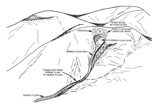
Figure 11-1. Debris may begin to flow as a mass when it becomes wet.
