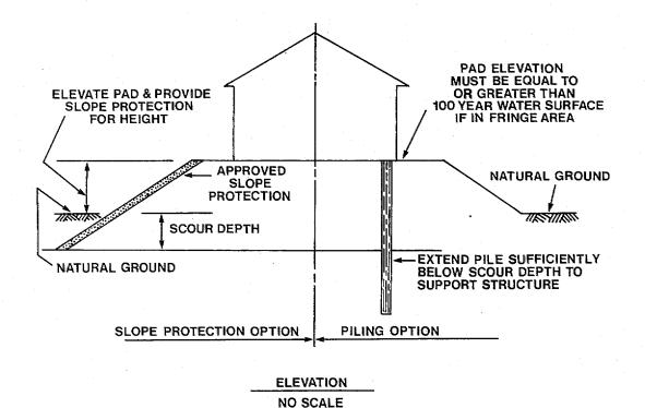
Figure 3-5: Suggested floodproofing criteria for structure in alluvial fan area. Source: Riverside County Flood Control and Water Conservation District's Cabazon Flood Study.
