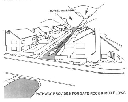
Figure: 11-4. Design and construction standards can be applied to reduce risk to structures.
