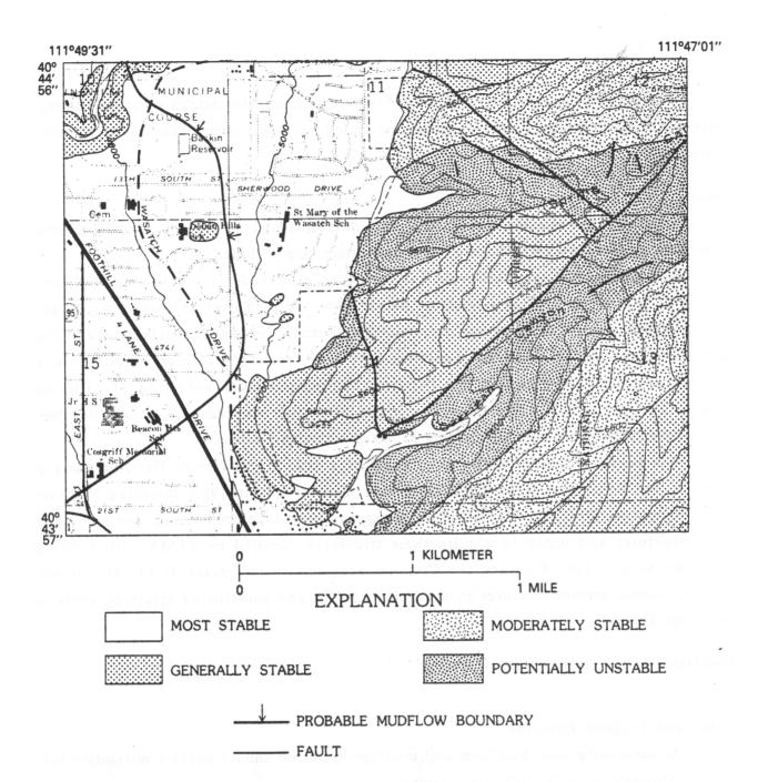
Figure 11-3. Mudslide susceptibility near Salt Lake City, Utah. "The features considered in preparing the relative slope stability map include: steepness of slope, type of rock or surficial deposit, and locations of bedrock, faults, springs, and former marshes. These features were evaluated according to their relation to known landslide deposits and talus accumulations, to the observed deterioration of buildings in the area, and, in small part, to plausible predictions." Source: U·S.G.S
