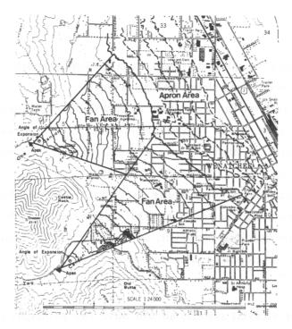
Figure 3-3. Topographic characteristics of typical alluvial fans and alluvial aprons (Wenatchee, Washington). Source: FEMA.
