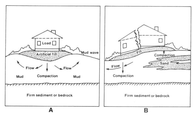
Figure 9-5. Damage due to differential compaction of soils. In A, soils have settled homogeneously. In B., the presence of the sand body results in differential settling with subsequent structural damage to the house. Source: U.S.G.S.
