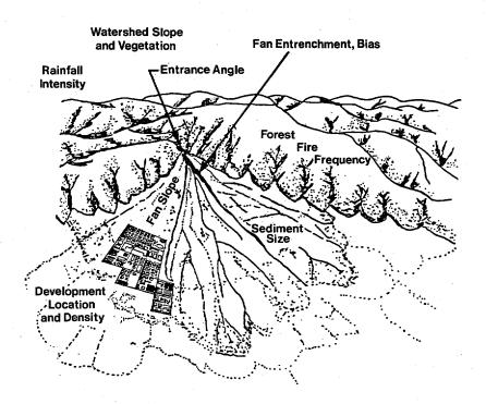
Figure 3-2. Factors affecting flood hazards on alluvial fans.
