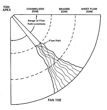
Figure 3-1. Hydraulic zones on a typical fan. Source: FEMA.
