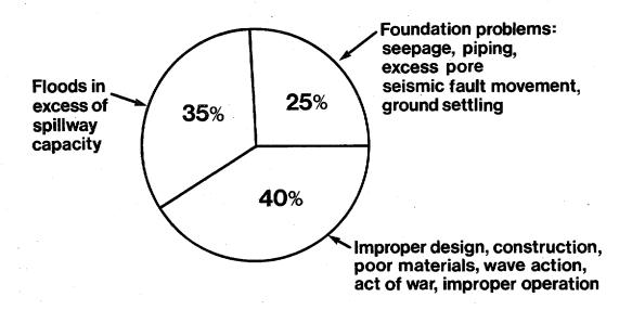
Figure 5-2. Causes of dam failure.
