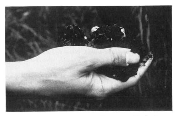
Figure 9-2. Organic soils like these are easily compressed, leading to subsidence. Source: unknown.
