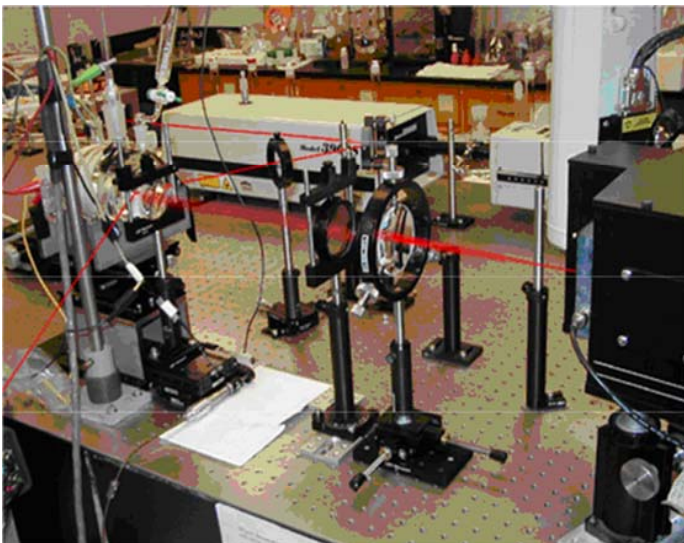
Surface Enhanced Raman Spectroscopy (SERS) – The electrochemical cell containing the sample under investigation (e.g. Alloy 22) by SERS.
