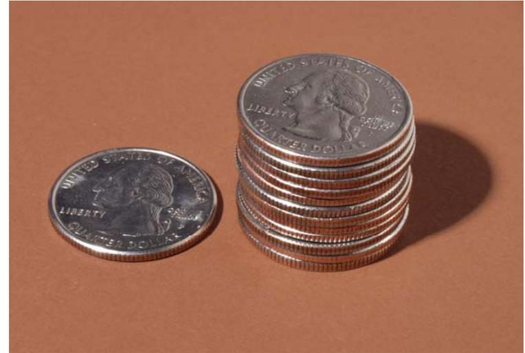
*16,000 to 160,000 years to penetrate the thickness of one U.S. Quarter for a corrosion rate of 0.1 to 0.01  $\mu\text{m}/\text{yr}$ .*
