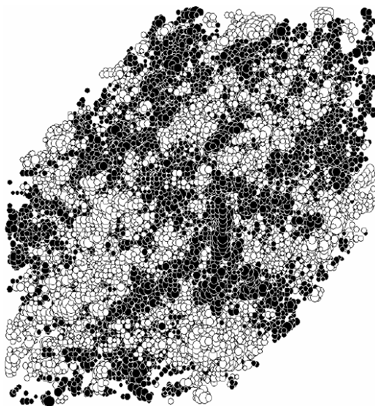
Figure 33 Energy landscape for an organic film with correlated disorder in a cubic lattice. White (black) circles correspond to hopping sites with energy above (below) the average hopping site energy. Dipoles are randomly distributed over the lattice. Since the energy landscape seen by any one charge depends on the locations of the other charges, the charge hopping rate cannot be assumed to be constant. [Novikov 2003]
