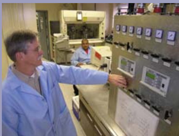
Ken Champagne, foreground, an engineering technician, and Mac Gray, background, a scientist in NETL's Office of Research and Development, test a sorbent developed at NETL to determine how well it captures carbon dioxide. (Source: NETL)
