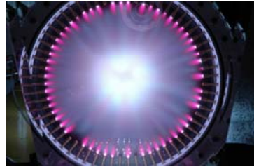
Fig. 3.4 Convergence of plasma jets to form an imploding plasma liner. (Witherspoon et al. 28 )
