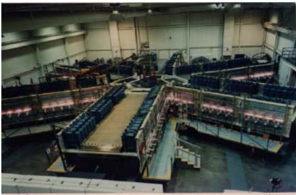
Figure 3.2 The Shiva-Star pulsed power facility is capable of delivering 12 MA in 10 \mu s for single-shot integrated MIF experiments.
