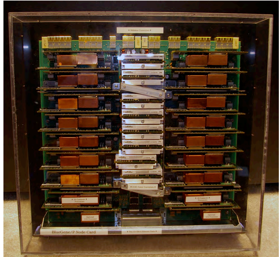
Blue Gene/P Node Card Prototype 32 Compute Processors 2 I/O Processors 2 10-Gb/s Ethernet Ports
