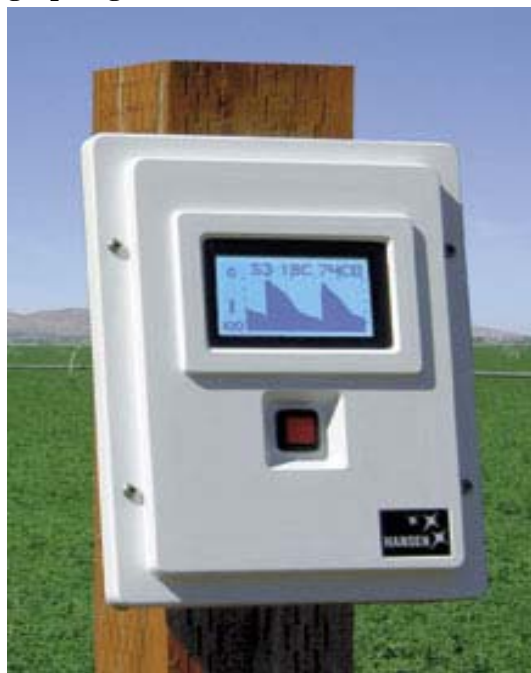
Figure 14, Soil moisture data recorder with graphing
