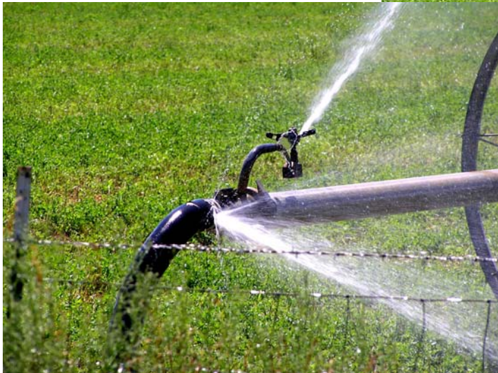
Figure 21, Hose leaks are rare but prolific and expensive to repair
