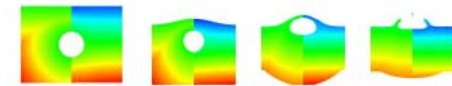
FIGURE 2 The new model allows predictions of the velocity (left side) and pressure (right) when a single gas bubble floats through a fluid to a free surface and bursts.
