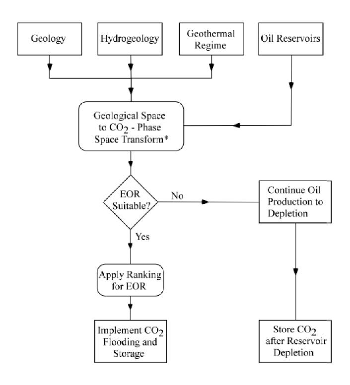
Figure 1: Diagrammatic representation of the process of screening and ranking of oil reservoirs for CO<sub>2</sub> - flood EOR and CO<sub>2</sub> storage (\* for details see Bachu, 2001b)
