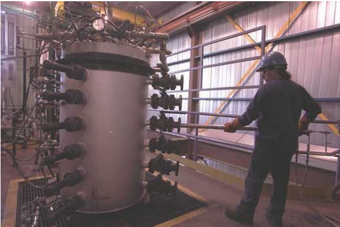
Figure 2 – Vertical Combustor Probing Access in Near Flame Region
