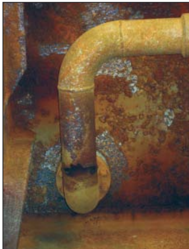
Figure 3: The "holed" fuel tank vent line in the number two cargo hold. USCG photo.
