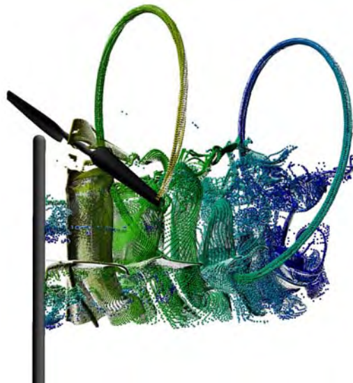
Figure 1: Unsteady Aerodynamics Experiment modeled with computational fluid dynamics, showing the wake from the turbine tower and the vortex from a blade tip. (Graphic courtesy of Fredrick Zahle, Risø National Laboratory)
