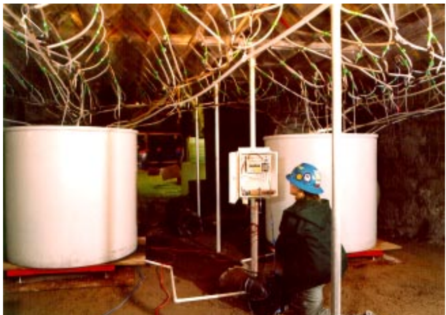
Conducting a seepage test in Alcove 1
