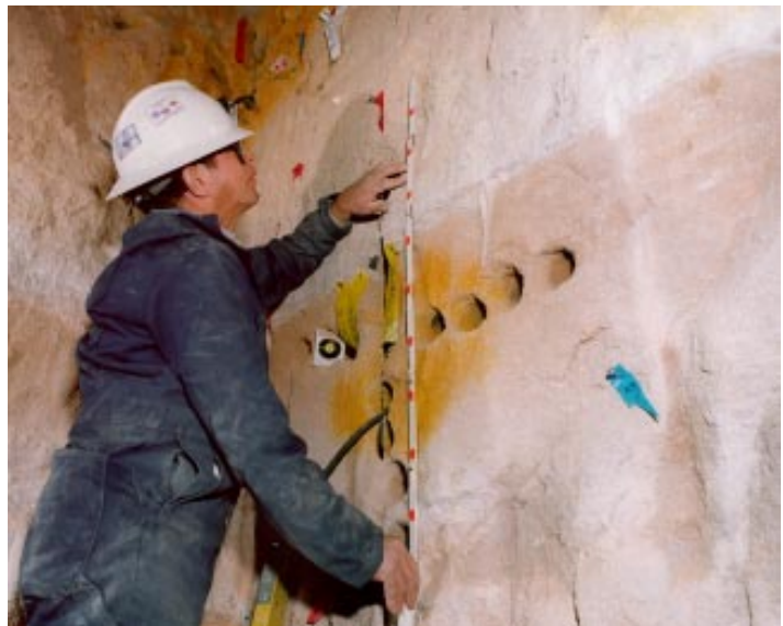
Preparing for a test using tracer elements to study rock properties
