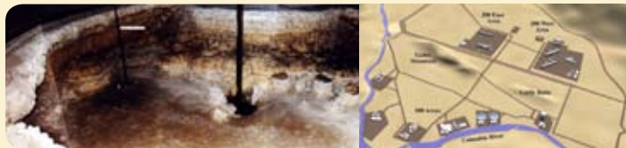
Saltcake is shown inside single-shell tank 105-B located at the Hanford Site in eastern Washington State.
