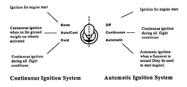
Figure 1. Typical Ignition Switch Position Labeling in TPE331-powered Airplanes
