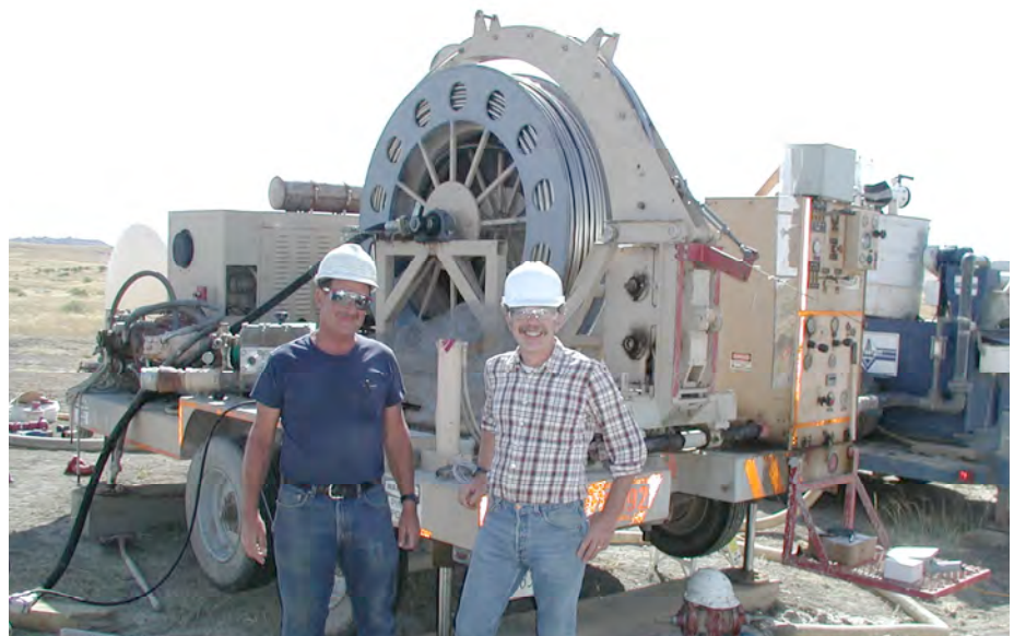
David Anderson (left) and Mike Fehler (right), LANL Geophysics Group Technician and Group Leader, respectively, on a Teapot Dome microwell drilling location with the LANL coiled tubing unit in the immediate background and the blue mud-cleaning unit behind the coiled tubing unit.
