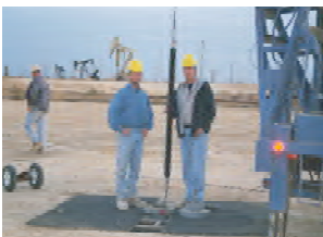
Crosswell receiver being prepared to lower in wellbore.
