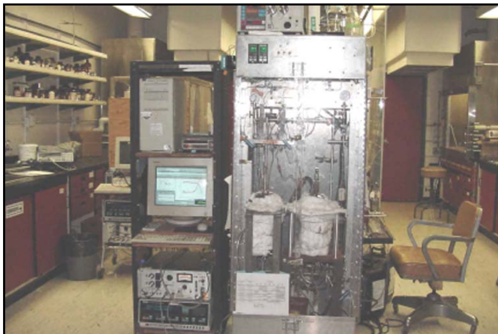
Figure 1. General view of the experimental system: supercritical test reactors and high-temperature loop, low pressure loop, and data acquisition system.
