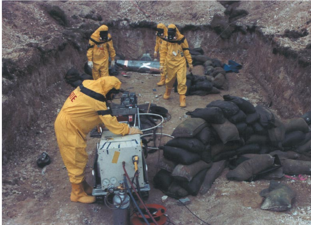
Specialized techniques, such as radiography, are used to examine the weapon's internal structure.
