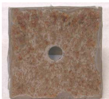
Original DAR40 After Exposure for 13 Cycles
