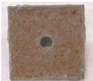
Type 316L Coating After Exposure for 13 Cycles
