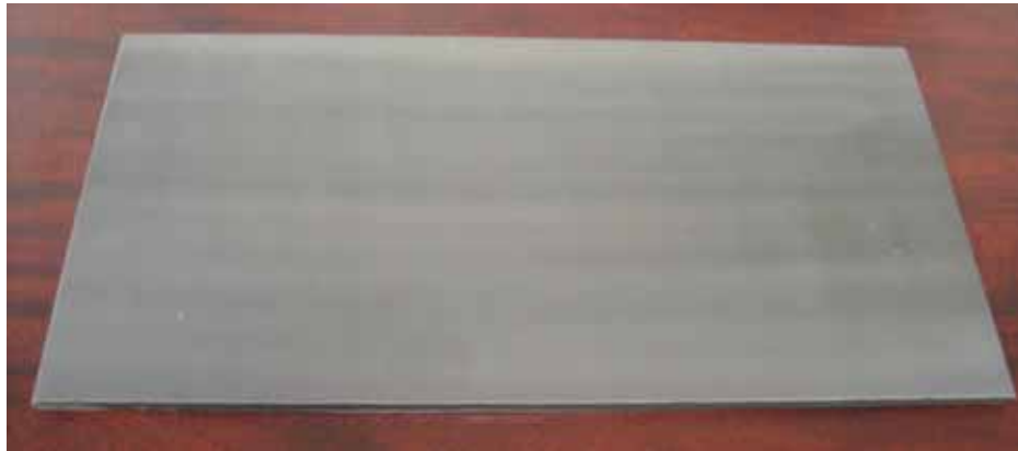
FIGURE 5. Thermal spray coated steel specimen (12" x 6" x 1/4").
