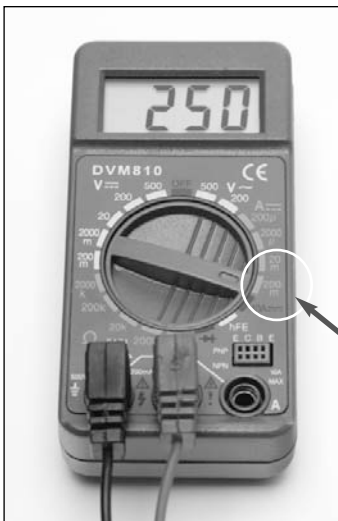
To measure amps for this fuel cell, set the dial at the 200m position.
