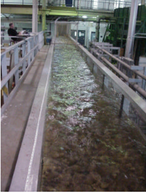
Figure 5 - View looking downstream in the 3 ft wide by 60 ft long by 1.5 ft deep adjustable slope flume.
