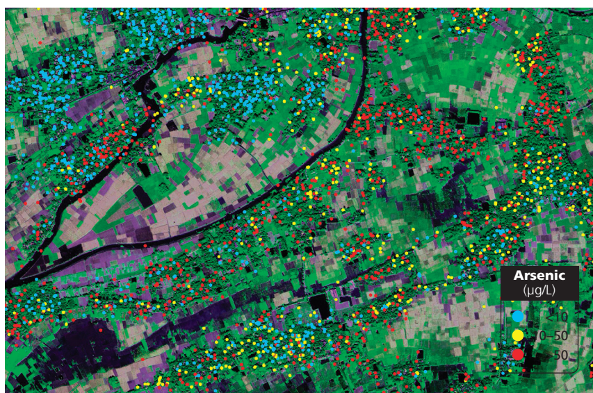
High-tech search for low arsenic. The Columbia project used GIS mapping (above) to survey arsenic concentrations in wells around Araihasar, Bangladesh. Safe wells are thusly labeled (right), and residents are encouraged to use them for drinking and cooking water.
