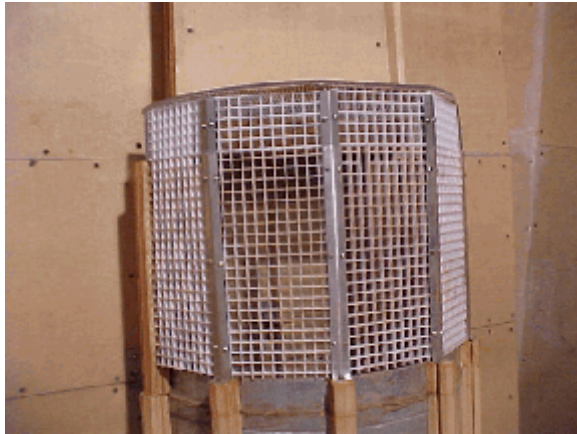
Figure 9. —Photograph of 25-ft-high trashrack (modification five).
