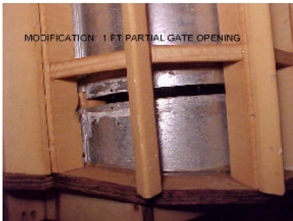
Figure 10. —Photograph of 1-ft gate opening with trashracks removed (modification six).
