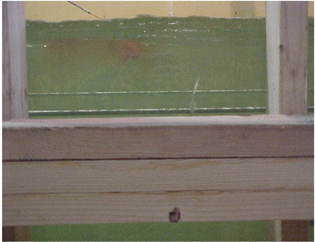
Figure 15. - Side view of dye tracing for the 220 hole diffuser with res. El. 1260, tailwater 970. Note the fiber tuft indicating an upward velocity component and the dye trace indicating a downstream movement with no strong recirculation patterns of turbulence. This photograph is similar to figure 14.
