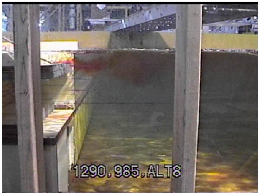
Figure 50. - Bottom dye injection for reservoir El. 1290 and tailwater El. 985.
