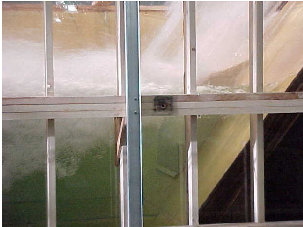
Figure 24. - Typical jet trajectory for the upper outlets operating at maximum reservoir El. 1290 and tailwater El. 958.
