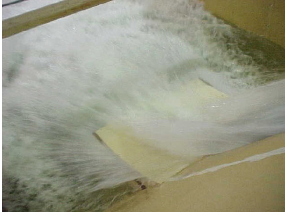
Figure 19. - Typical flow pattern and jet trajectory for the mid-level outlets operating at minimum reservoir El. 1208 and tailwater El. 958.
