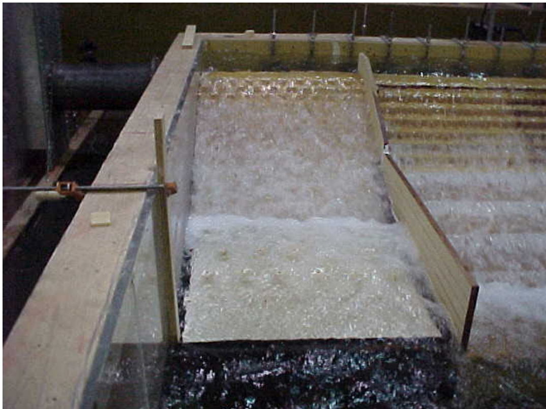
Figure 42. - Baffled apron over the 2:1 sloping cascade section with the baffled, adjustable horizontal basin and apron. The flow shown is the design flow with reservoir El. 1290 and tailwater El. 965.
