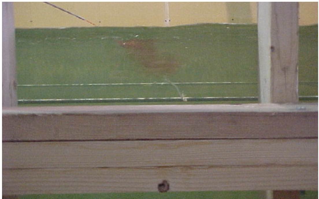
Figure 14. - Side view of outlet works operations with the diffuser under Res. El. 1260, tailwater 970 with flow from right to left. Minimal surface turbulence is observed. Fiber tuft indicates upward and slightly downstream flow direction. Dye indicating the same flow directions, upward and downstream.
