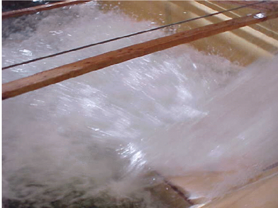
Figure 23. - Typical jet trajectory for the upper outlets operating at maximum reservoir El. 1290 and tailwater El. 958.
