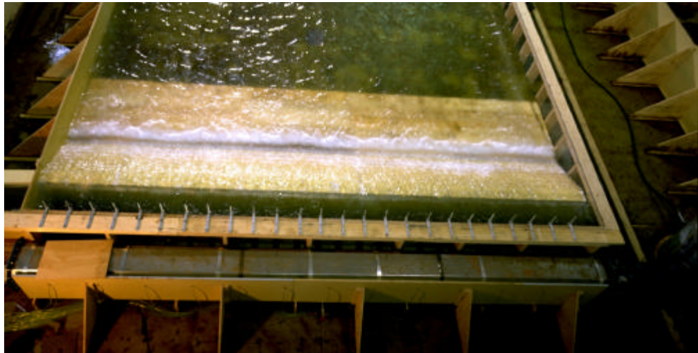
Figure 41. - Grand Coulee Dam forebay cascade model with the conceptual design for initial model study.
