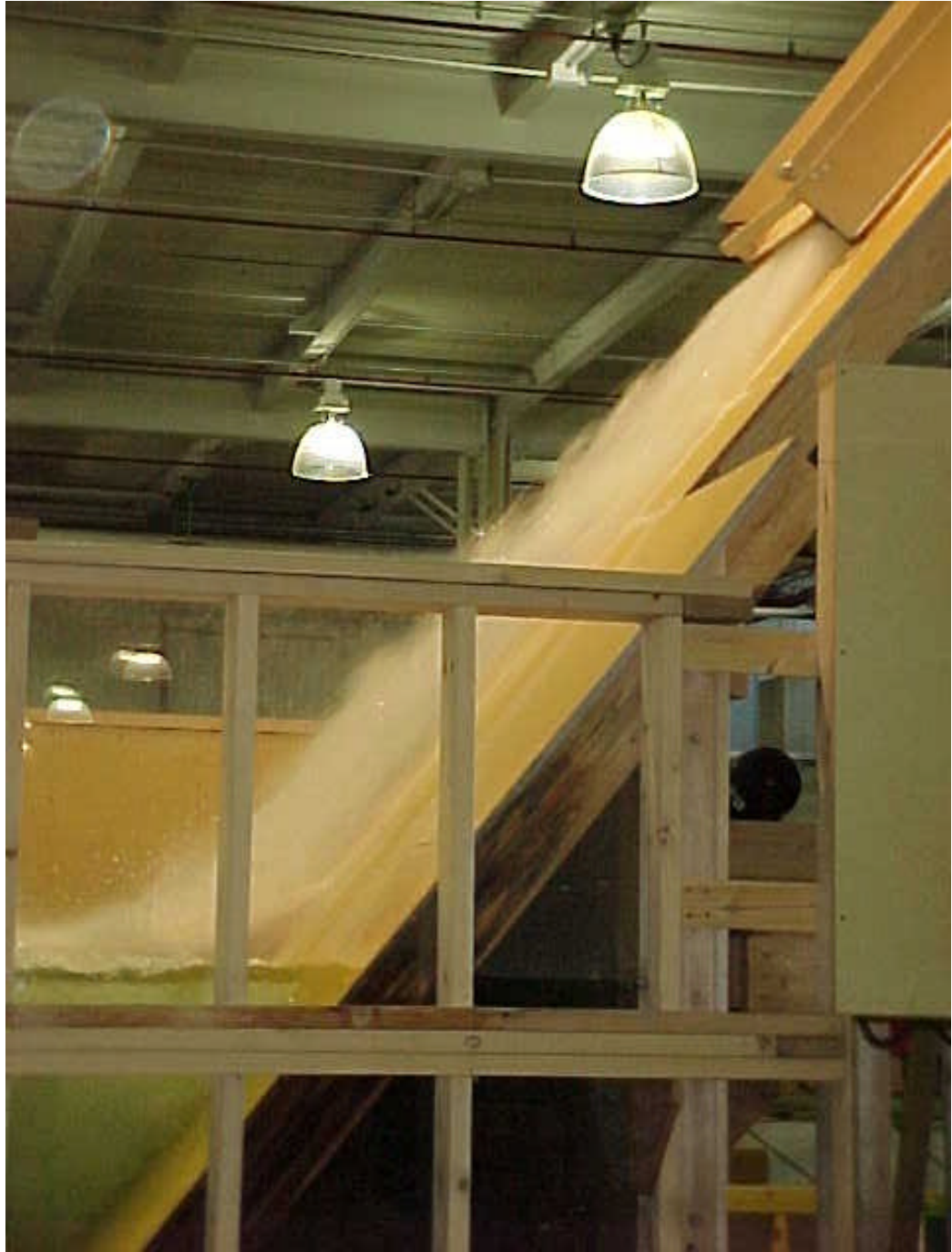
Figure 32. - Simulated spillway flow down the dam face and impacting on the deflector. Spillway discharges were more easily deflected than the outlet works discharges, behaving more similar to expected deflector performance.
