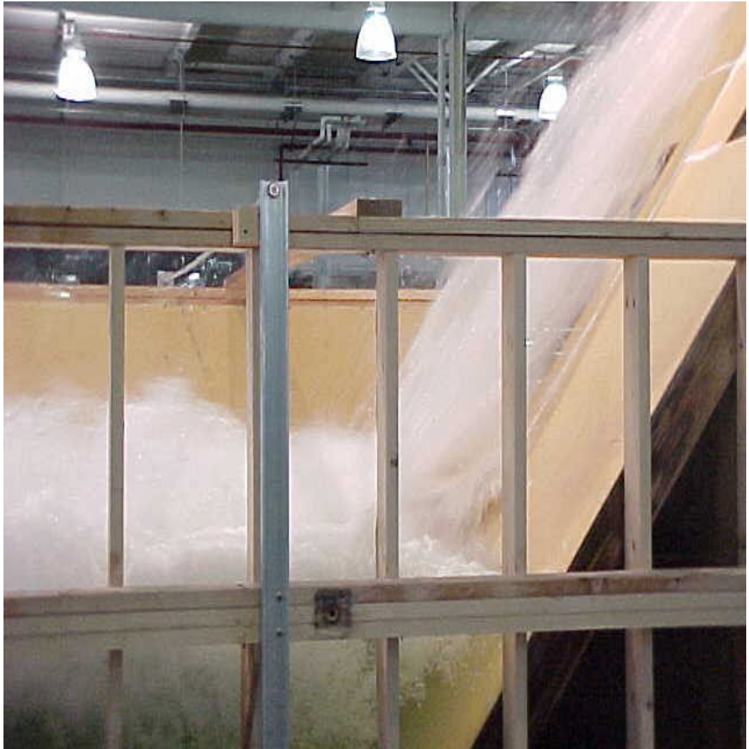
Figure 28. - Typical jet trajectory for combined outlets operating at maximum reservoir El. 1290 and tailwater El. 958.
