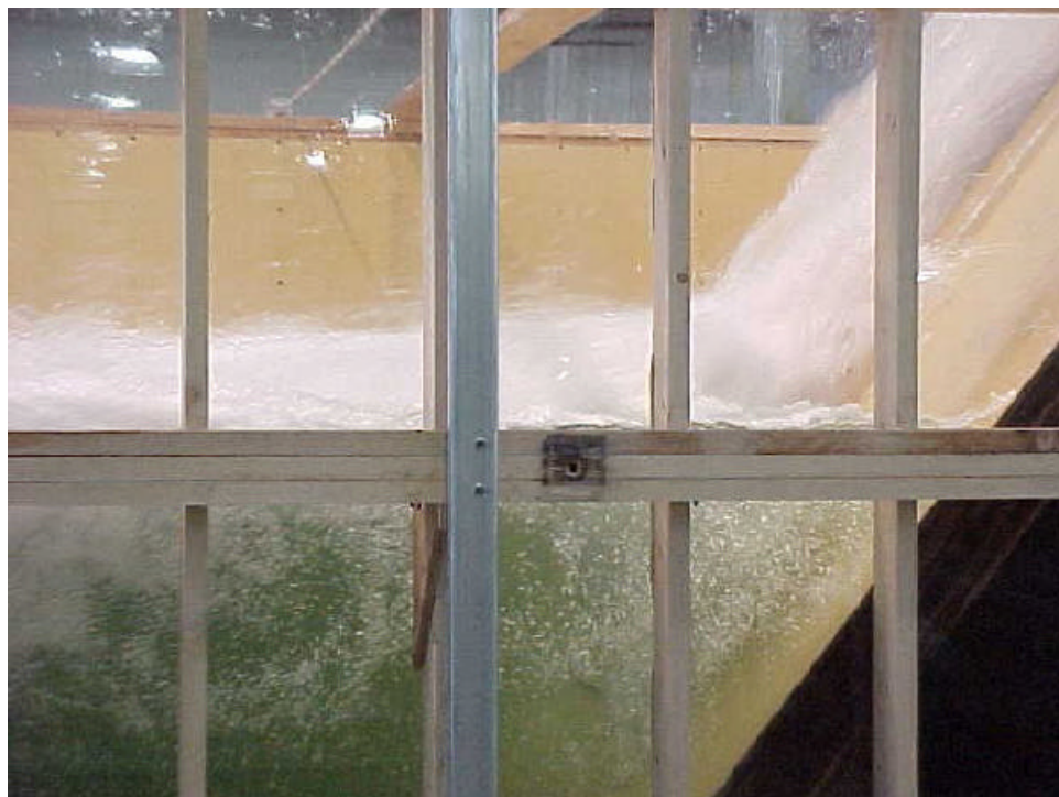
Figure 26. - Typical jet trajectory for combined outlets operating at minimum reservoir El. 1208 and tailwater El. 958.
