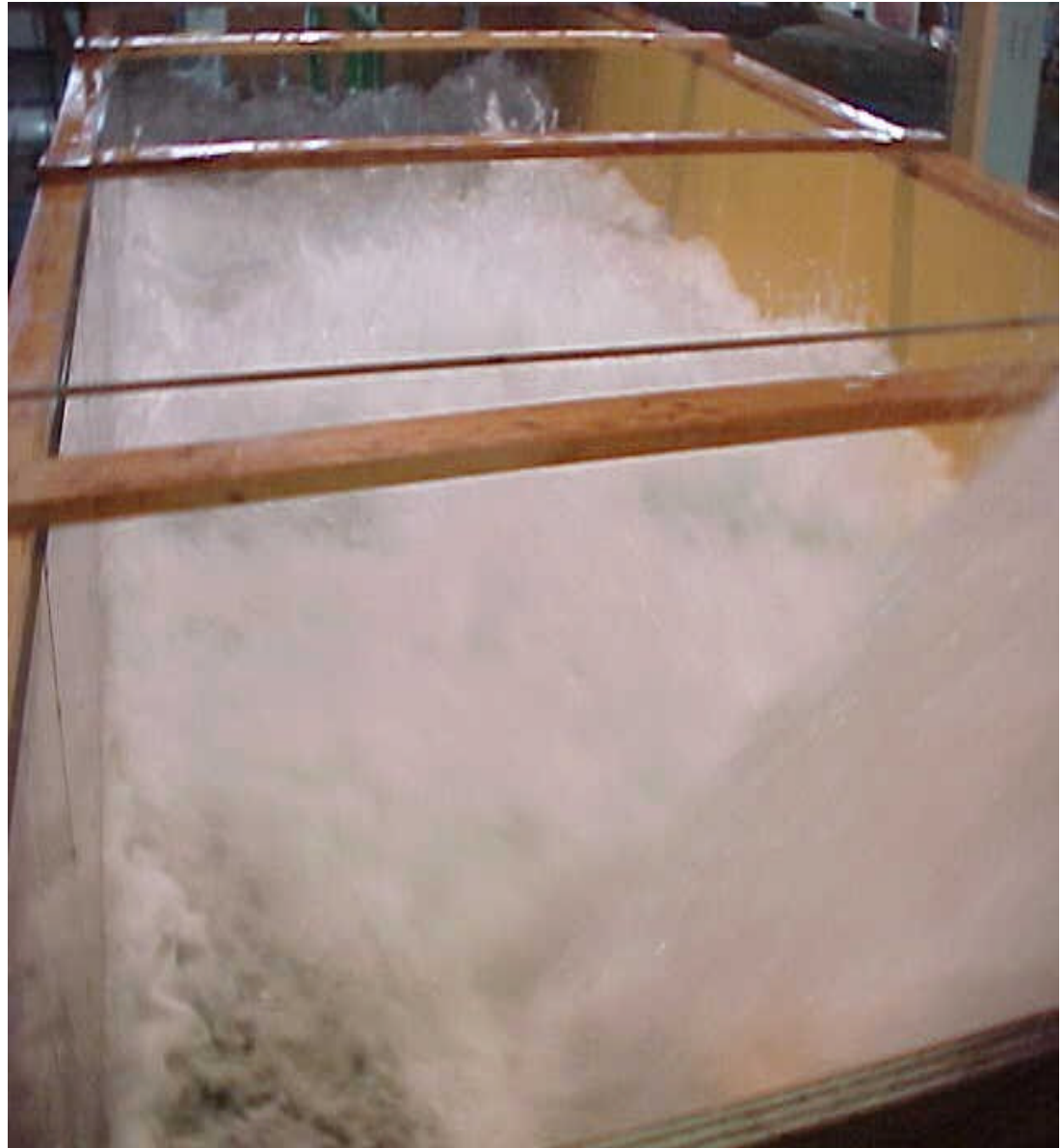
Figure 27. - Typical jet trajectory for combined outlets operating at maximum reservoir El. 1290 and tailwater El. 958.
