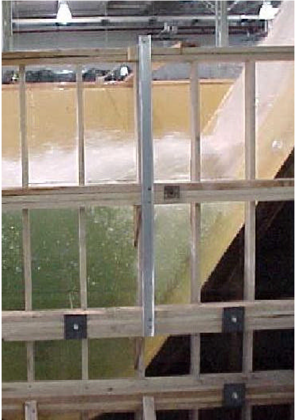
Figure 22. - Typical jet trajectory for the upper outlets operating at minimum reservoir El 1208 and tailwater El. 958.
