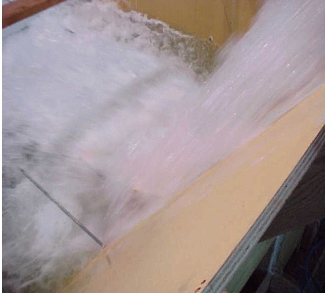
Figure 21. - Typical jet trajectory for the upper outlets operating at minimum reservoir El. 1208 and tailwater El. 958.
