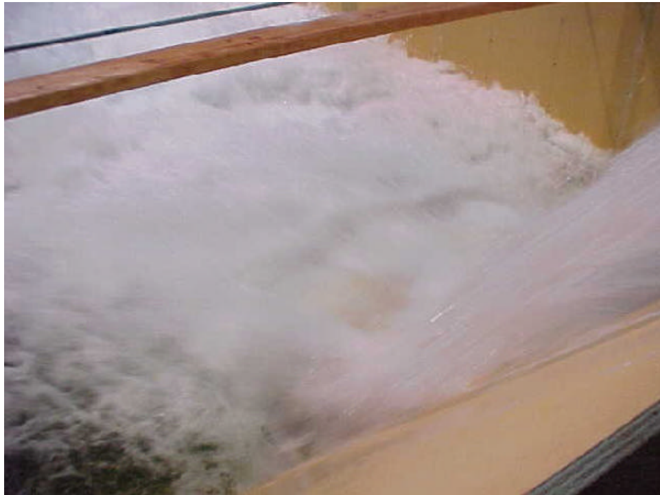
Figure 25. - Typical jet trajectory for combined outlets operating at minimum reservoir El. 1208 and tailwater El. 958.
