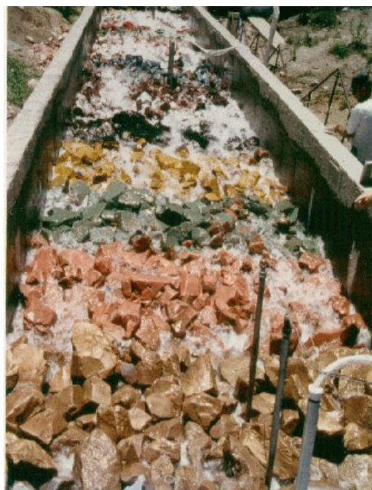
Figure 3. - Overall view, looking down the slope, of the 1997 riprap material with q=0.09 \text{ m}^3/\text{s}/\text{m} . The pipes extending through the riprap were used to measure interstitial velocities. (Fig3.bmp)
