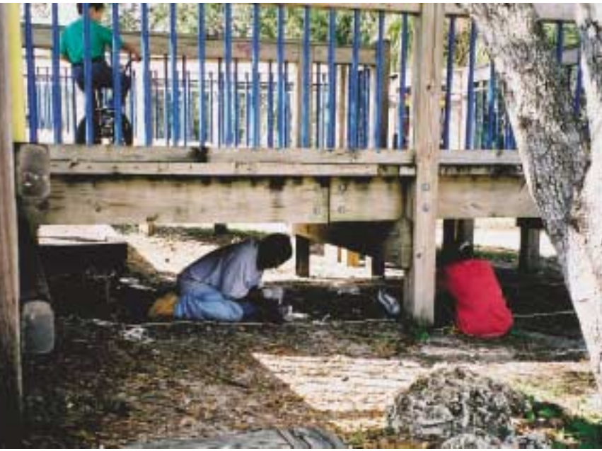
Under the boardwalk. University of Florida students measure arsenic under CCA-treated wood structures to gauge the extent to which the metal leaches from treated lumber. Although the chemicals in CCA are largely fixed in treated wood, problems arise when the lumber degrades or is burned at the end of its usefulness. The length of the service life of CCA-treated wood is debated, but most experts agree that an influx of the material will soon hit the waste stream.
