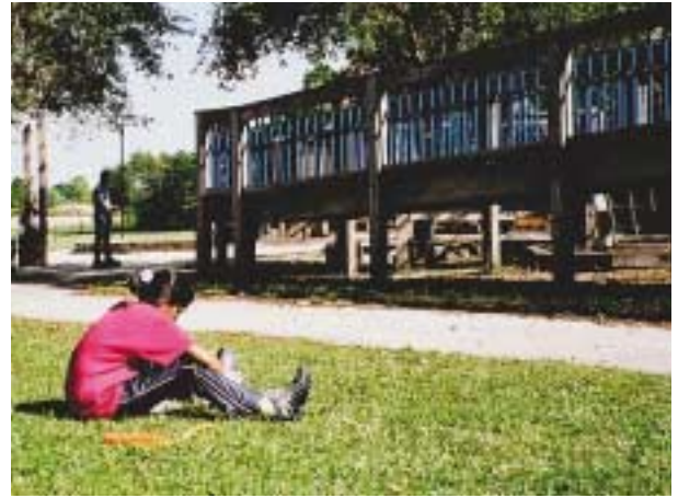
Under the boardwalk. University of Florida students measure arsenic under CCA-treated wood structures to gauge the extent to which the metal leaches from treated lumber. Although the chemicals in CCA are largely fixed in treated wood, problems arise when the lumber degrades or is burned at the end of its usefulness. The length of the service life of CCA-treated wood is debated, but most experts agree that an influx of the material will soon hit the waste stream.
