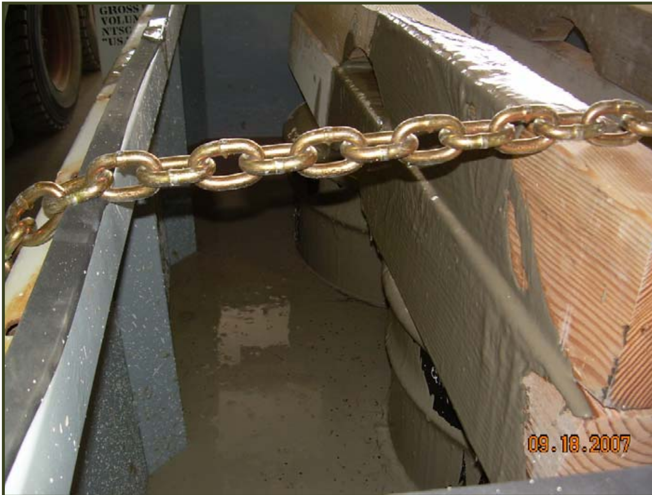
Mixed Waste Drums Encapsulated in a B-25
