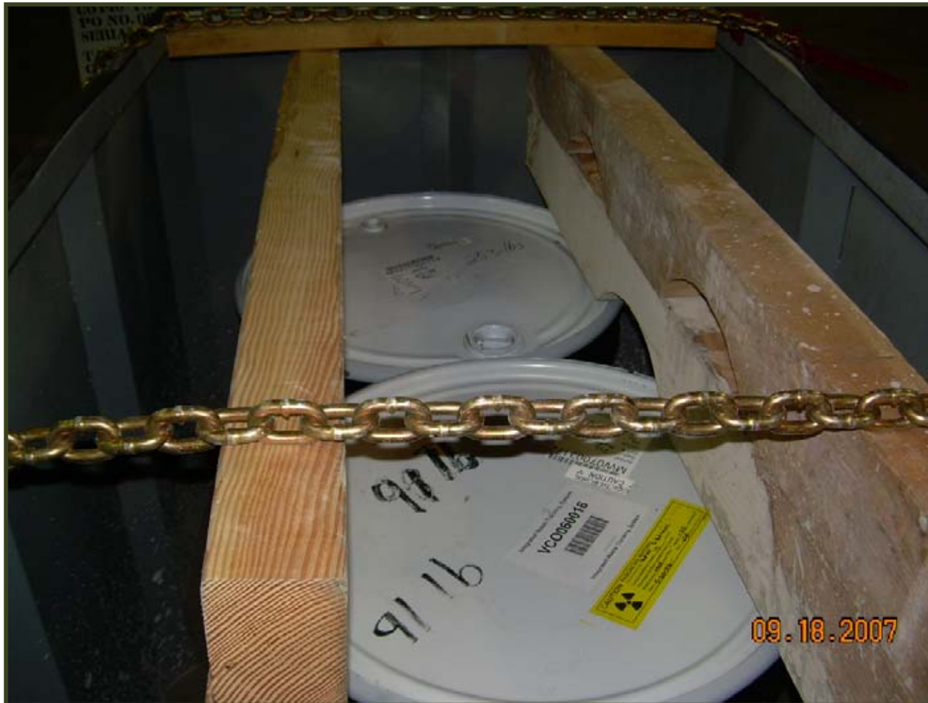
Mixed Waste Drums Encapsulated in a B-25
