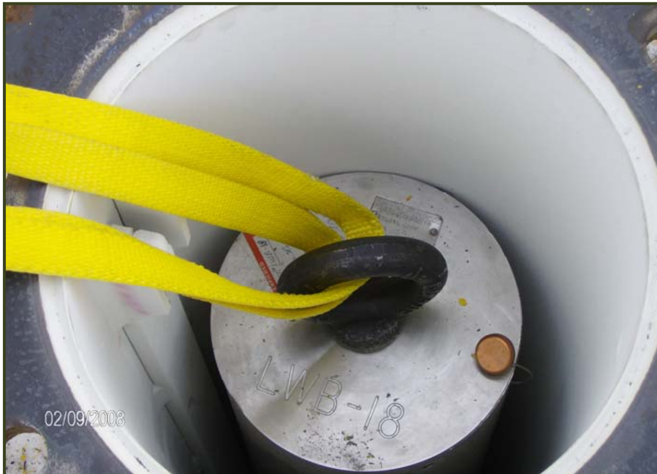
Unirradiated Light Water Breeder Reactor (ULWBR) Fuel Packaging for Transport to the Nevada Test Site
