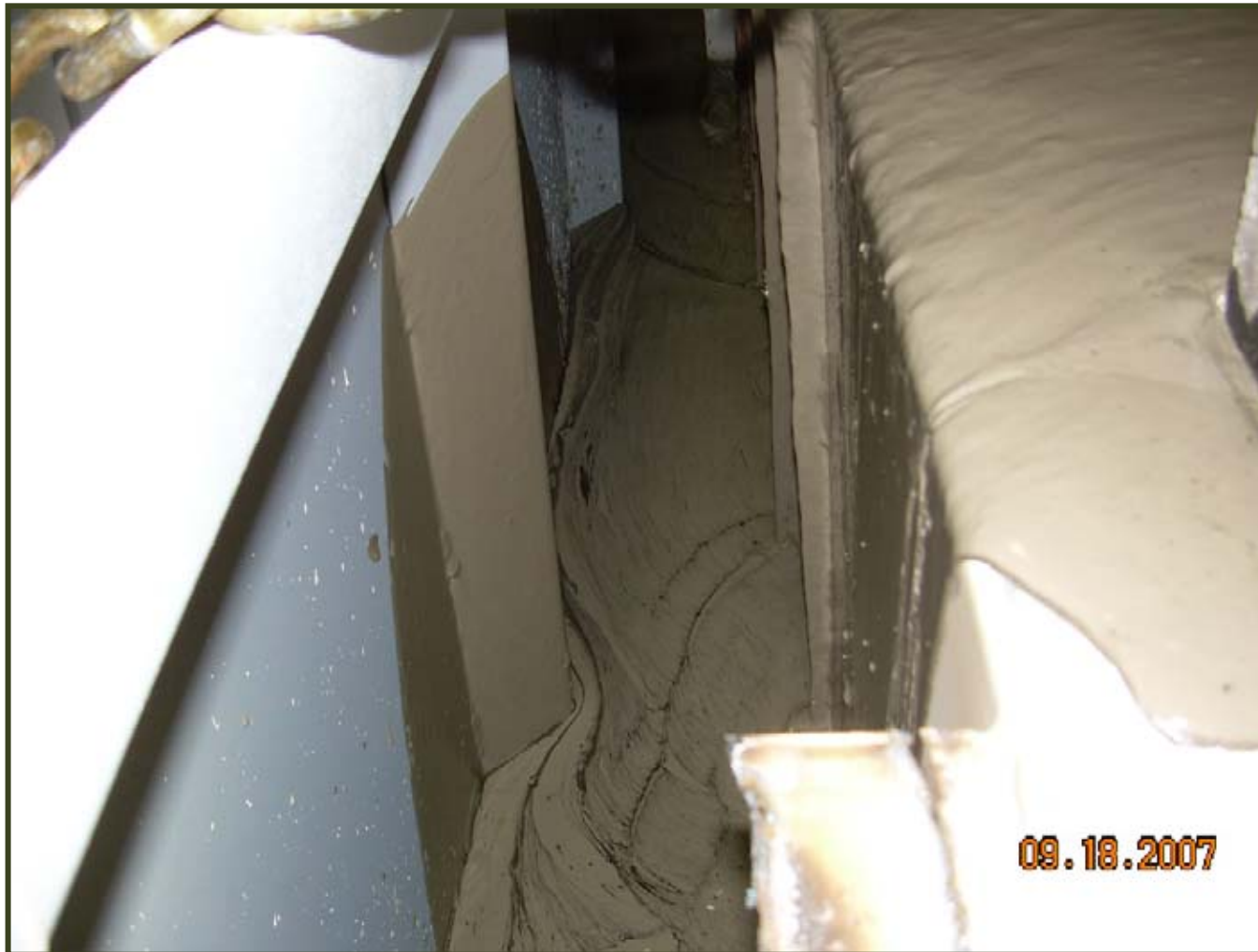
Mixed Waste Drums Encapsulated in a B-25
