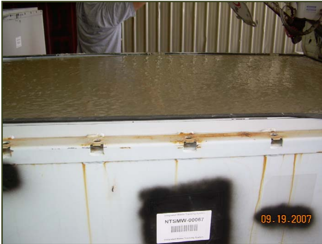
Mixed Waste Drums Encapsulated in a B-25
