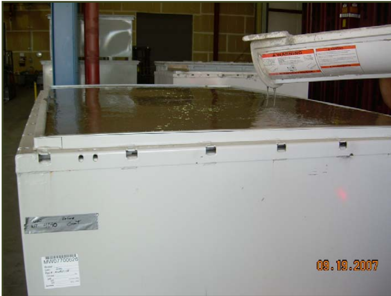
Mixed Waste Drums Encapsulated in a B-25
