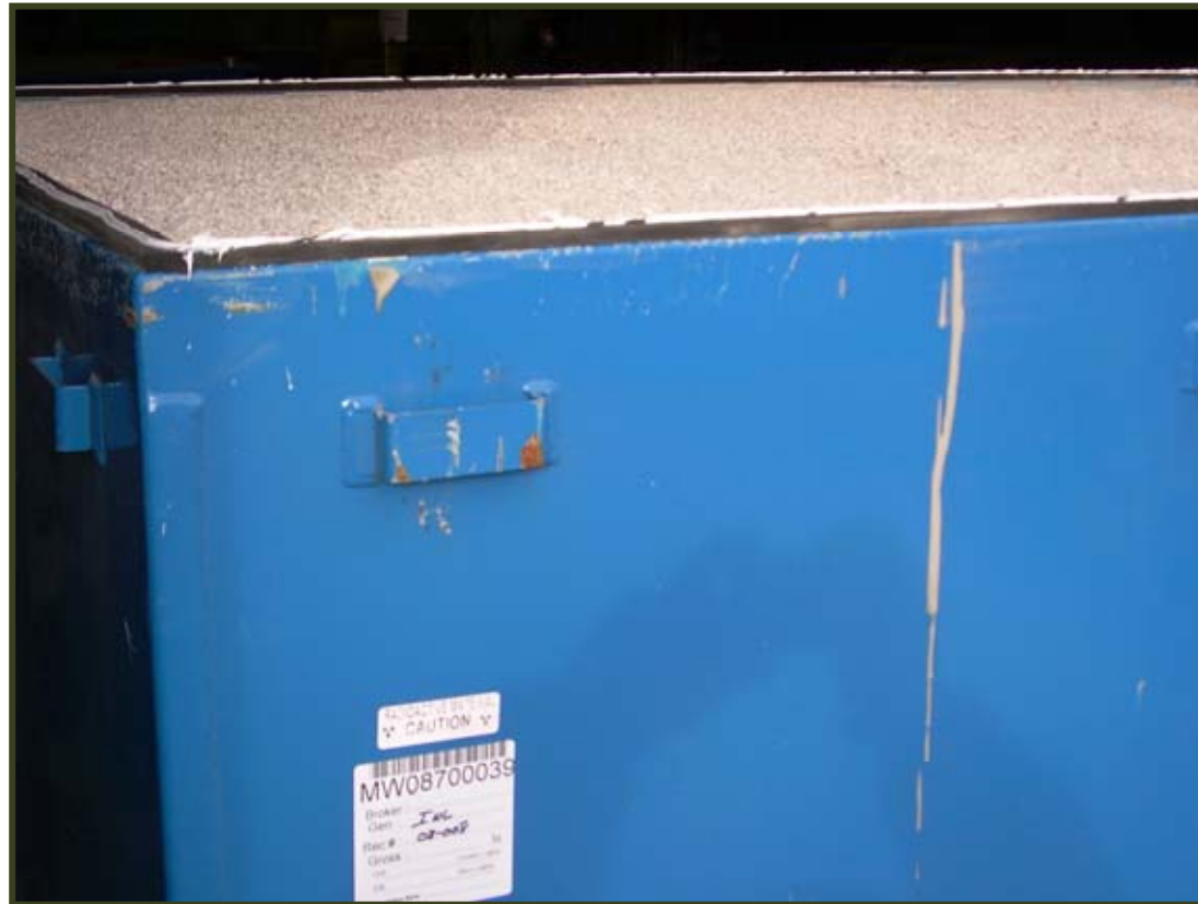
Cured grout box filled with absorbent
