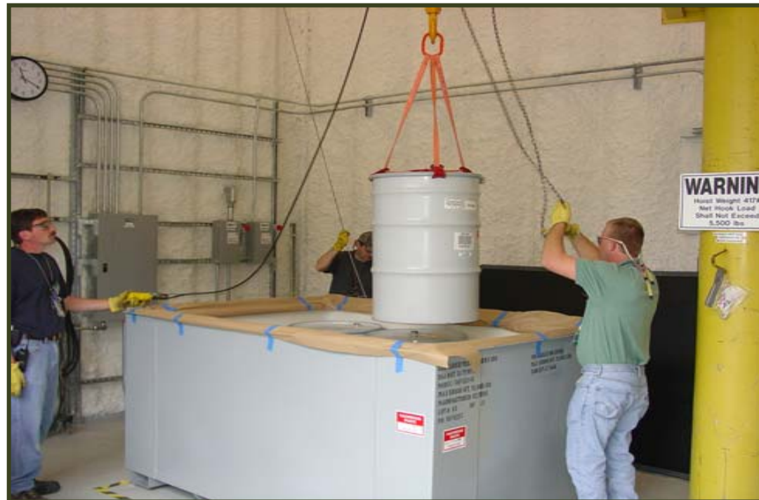
Waste drums loaded into UltraTech box
