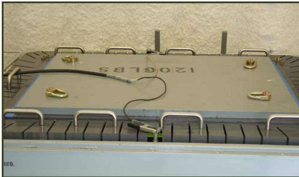
Macro Liner lid being fused to macro liner
