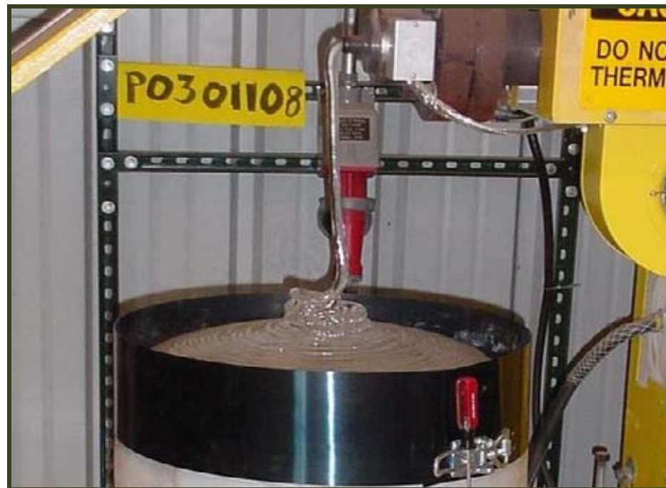
Heated LDPE poured around debris
