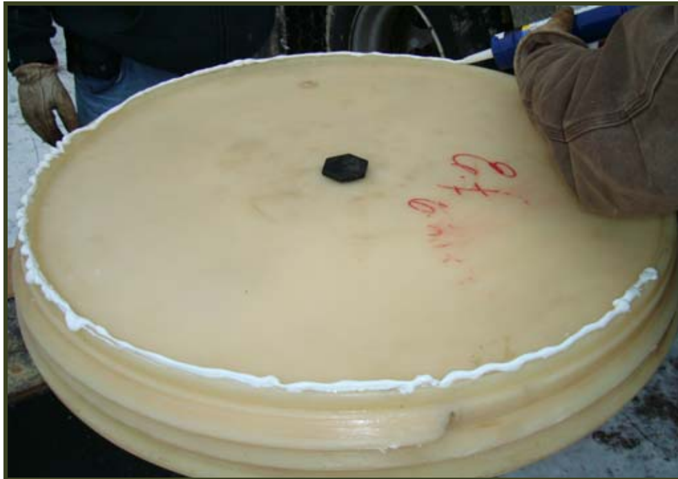
Epoxy applied to HIC lid
