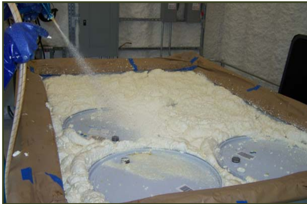
Loaded box sprayed with foam to fill void space
