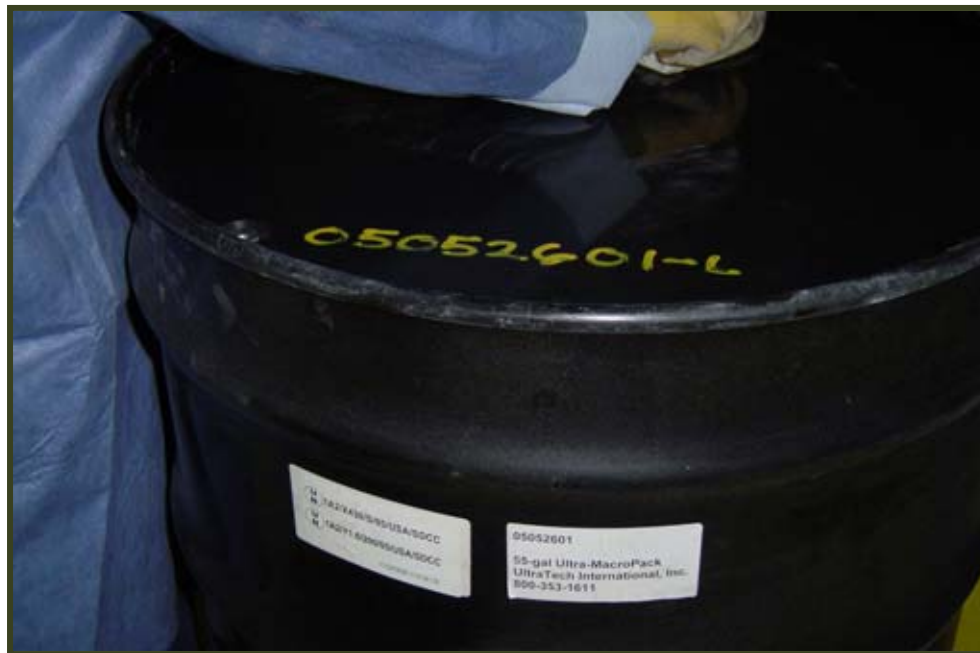
Closing 55-gallon Macro Liner container
