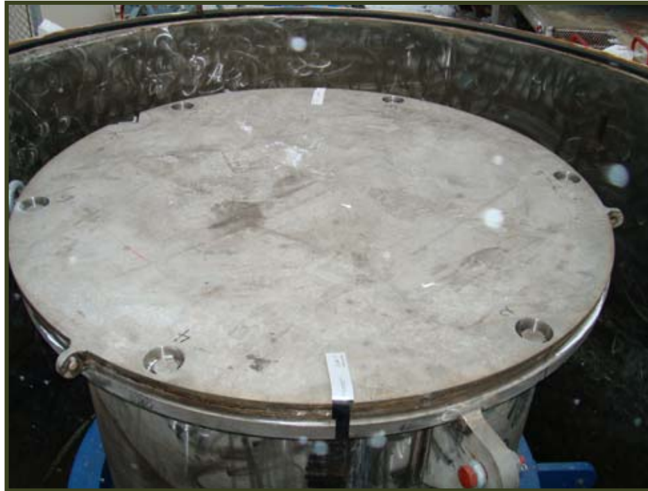
Final package after emplacement in shipping cask
