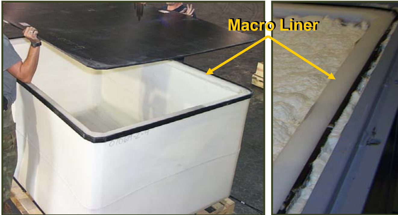
Poly liner in steel box
