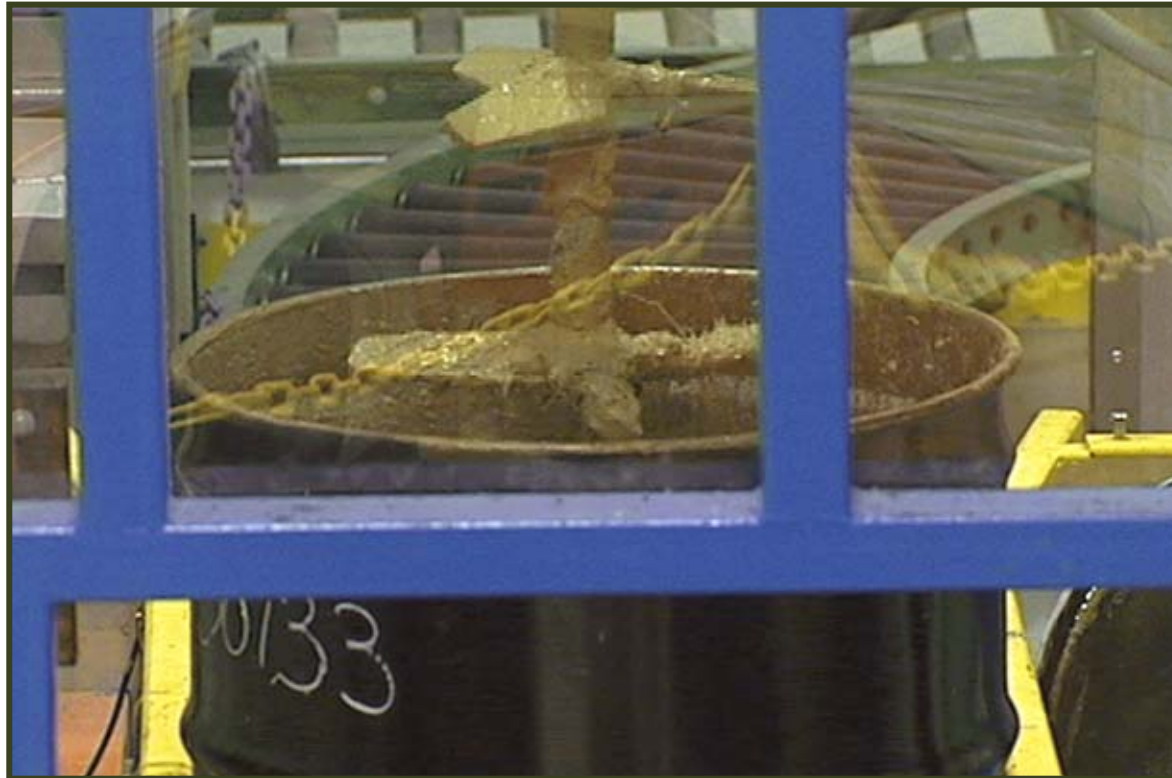
Stabilization using mixing blade in drum
