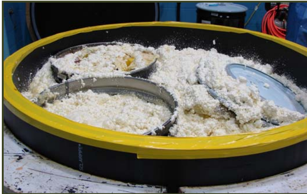
UltraTech 63-inch diameter MacroPack loaded with debris and foam to fill void space
