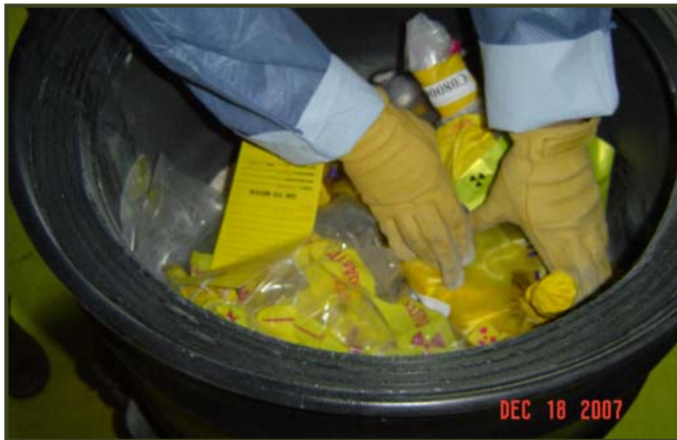
Debris waste being loaded into 55-gallon UltraTech Macro Liner container
