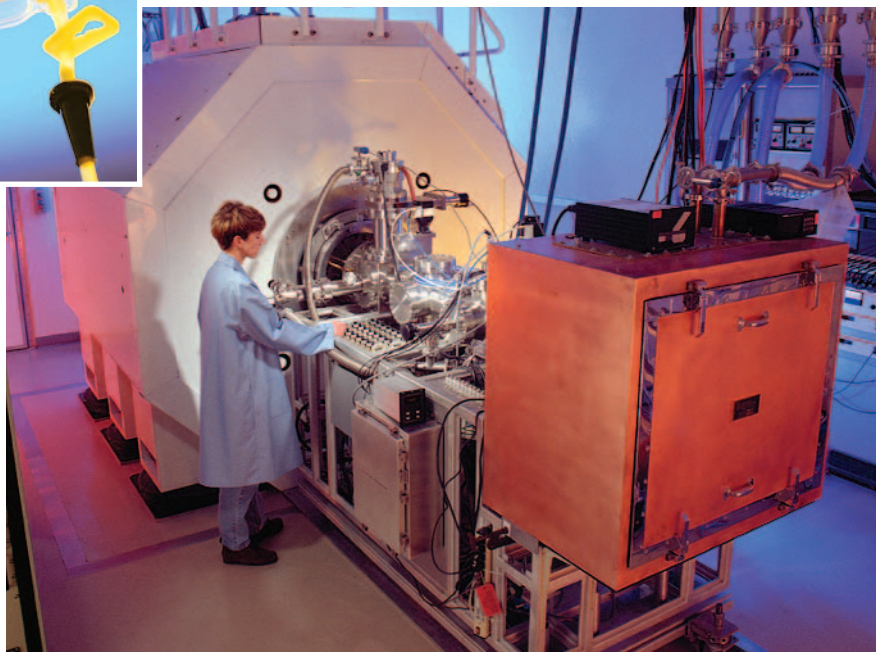
Big picture, tiny molecules. A PNNL researcher performs an experiment on the Fourier transform ion cyclotron resonance mass spectrometer, which is used to characterize proteins such as those in blood plasma (inset).
