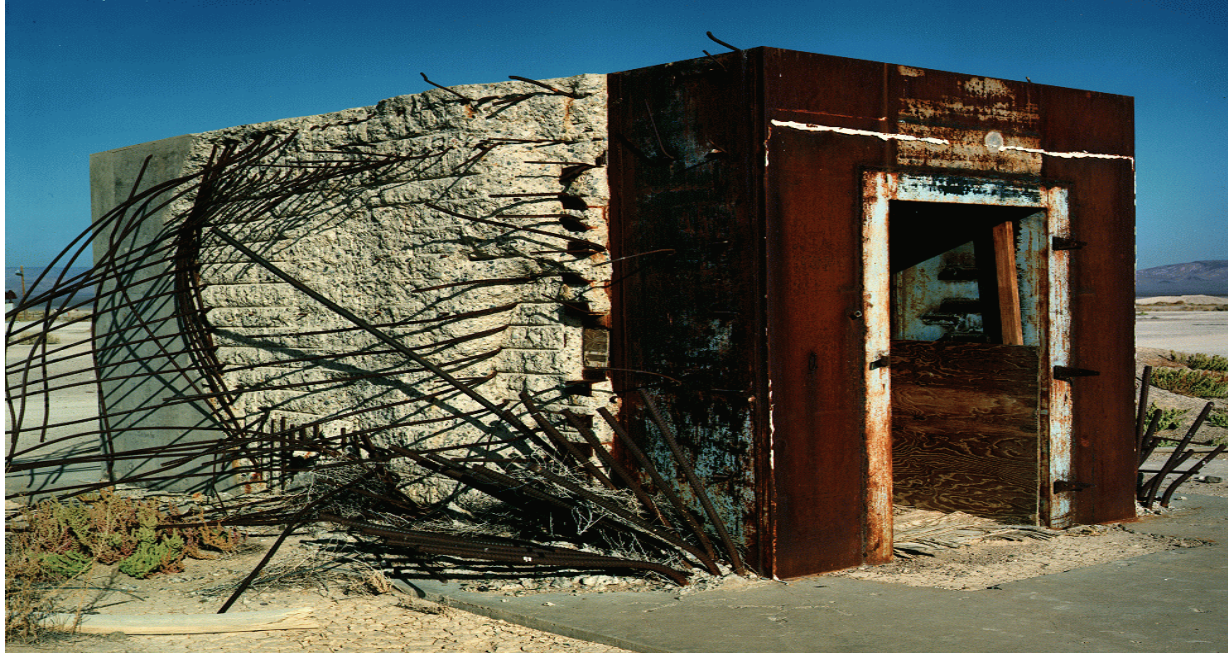
Mosler bank vault. Bottom left photo shows the vault prior to the 1957 Priscilla test. The above and bottom right photo show the effect of the blast on the vault directly after the test.
