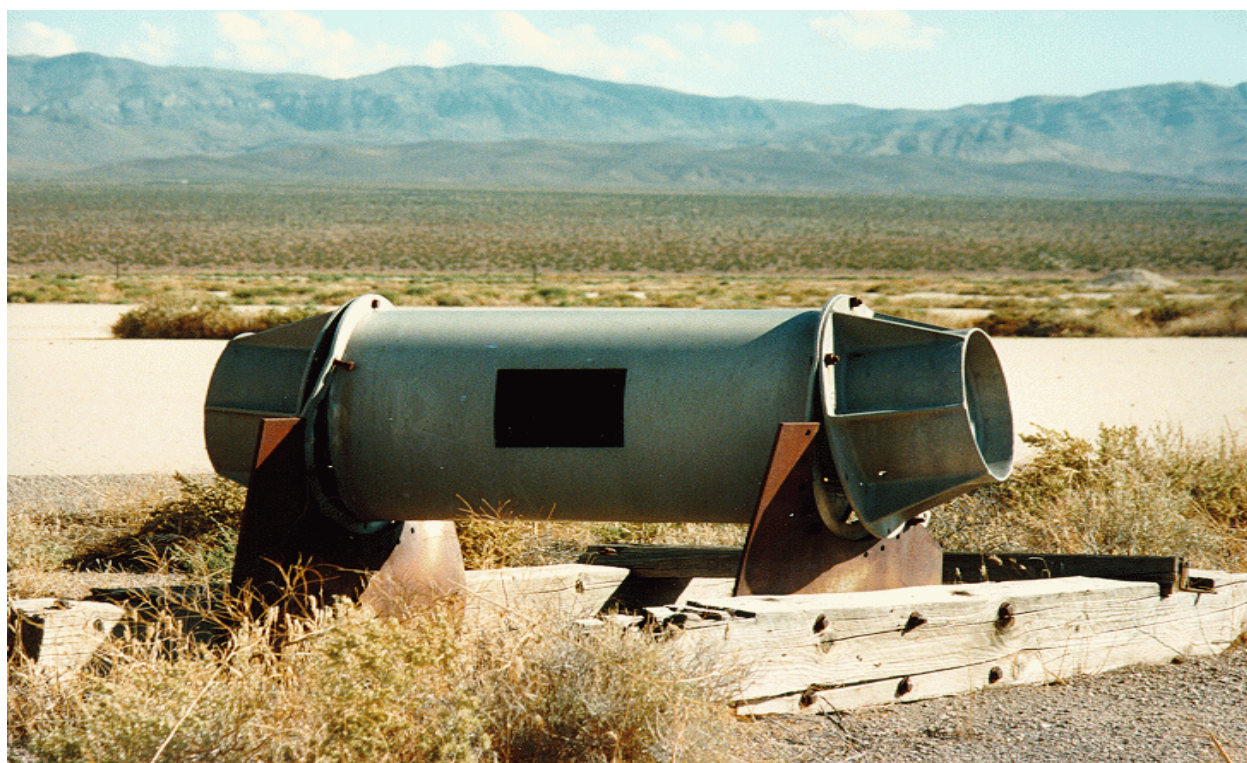
For the Encore test, 11 pigs were placed in cylindrical aluminum containers with fabric-covered portholes. Altogether there were three stations located on Frenchman Flat.
