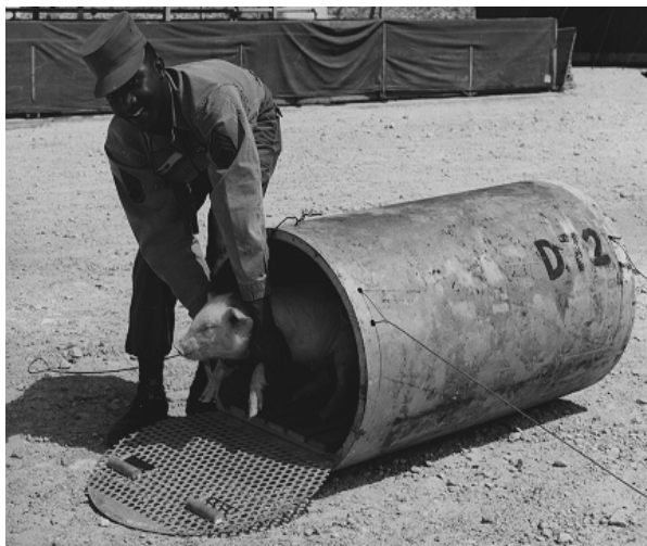
A 25-pound shoat is removed from an aluminum barrel by SSgt Nathaniel Morgan, 47th Field Hospital, Fort Sam Houston, Texas. The containers were positioned at various distances from ground zero to measure radiation doses.
