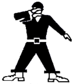
HOT BRAKES Fans face - Points to brake
