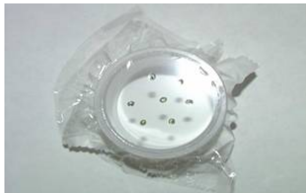
Dried Pu spotting technique (analysis by XRF through film)
