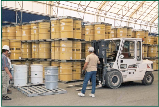
Workers transferred transuranic waste drums during the characterization process at the Nevada Test Site.
