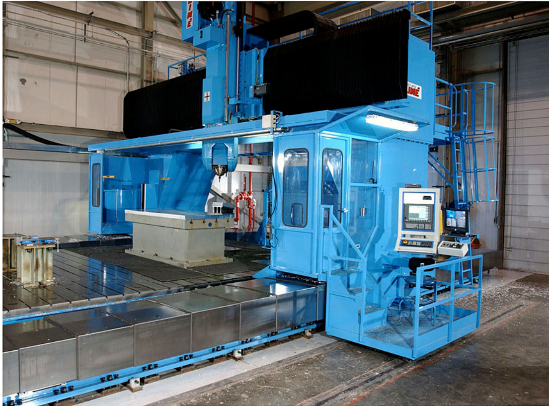
High-Speed Henri Liné 5-Axis Gantry Mill
